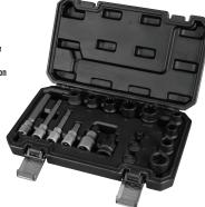
5 Point sockets: 10mm, 12.5mm, 14mm, 19mm 5 Point male bit socket: 10mm. 7 Point sockets: 14mm, 22mm. 10 Point sockets: 11.5mm, 15mm, 20mm. 6 Point male bit socket: 7mm stubby, 7mm std, 7mm extra-long, 8mm stubby. 6 Point male bit socket: 9mm stubby, 9mm extra-long, 11mm extra-long. 12 Point Tamper-Proof bit socket: 14mm.
